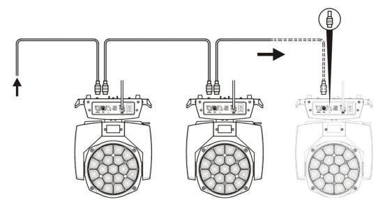
For installations where the DMX cable has to run a long distance or is in an electrically noisy environment, such as in a discotheque, it is recommended to use a DMX terminator. This helps in preventing corruption of the digital control signal by electrical noise. The DMX terminator is simply an XLR plug with a 120  $\Omega$  resistor connected between pins 2 and 3,which is then plugged into the output XLR socket of the last fixture in the chain. Please see illustrations below.
