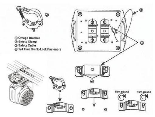
Regardless of the rigging option you choose for WashFX 300, always be sure to secure your fixture with a safety cable. The fixture provides a built-in rigging point for a safety cable on the hanging bracket as illustrated above. Be sure to only use the designated rigging point for the safety cable and never secure a safety cable to a carrying handle.
