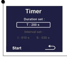
Using the adjustment wheel, place the cursor on the "Duration Set" information and click, you will now set the total operating time of the timer, the total time can be set from 1 second to 999 hours.
