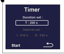
Using the adjustment wheel, place the cursor on the "Duration Set" information and click, you will now set the total operating time of the timer, the total time can be set from 1 second to 999 hours. Once the total duration information has been set, you can adjust the start & stop interval of your device.
